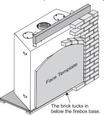
FPI offers a cover plate template. See the "Optional Cover Plate Template" section.
